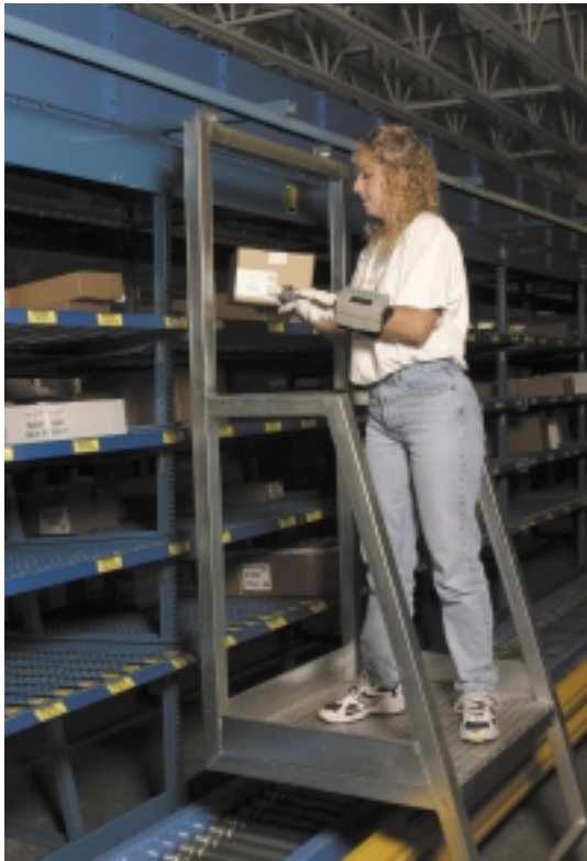
McKesson's integrator developed library-type ladders to allow employees to easily replenish the back of flow racks in the split-case pick area. The ladder crosses over a conveyor line below.
